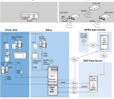
DC **Driver Card VST** VDO SmartTerminal latest generation of the download terminal DLD SR II **Download Device Short** TM VDO Fleet Tachograph Range II Management **DLD WR II** Download Device Wide **VDO Fleet Motion MOT** Range II R DL 4G Remote DL 4G MCR Mobile Card Reader DLK Download Key to transfer Tools · VDO Fleet Automatic driver card and mass Upload memory data **VDO Fleet Connect DLK Pro** New generation of the VDO Fleet Extract download key
